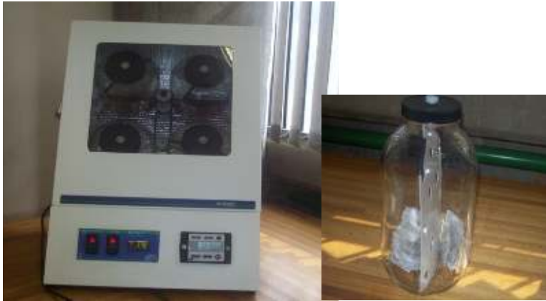
Figure 1 Ankom Daisy II incubator and fermentation jar with bags containing feed samples
