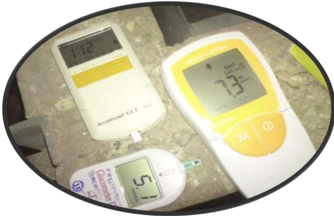
**Figure 1 Glucometer Elite, Accutrend GCT and Accutrend plus**
