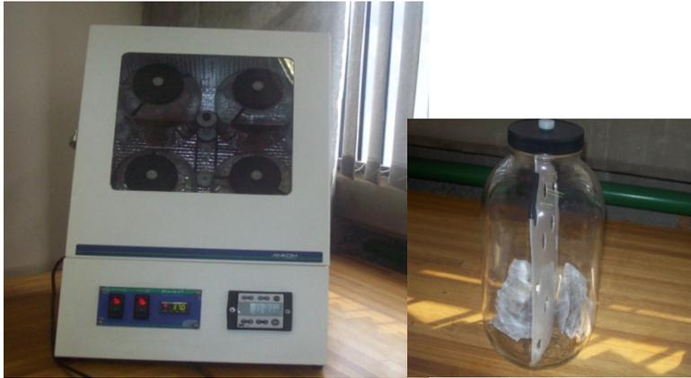
Figure 1 Ankom Daisy<sup>II</sup> incubator and fermentation jar with bags containing feed samples
